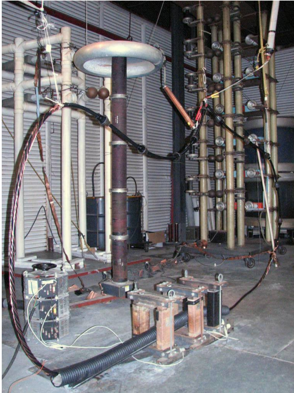
Figure 3: Set-up for impulse voltage tests at high temperature.
